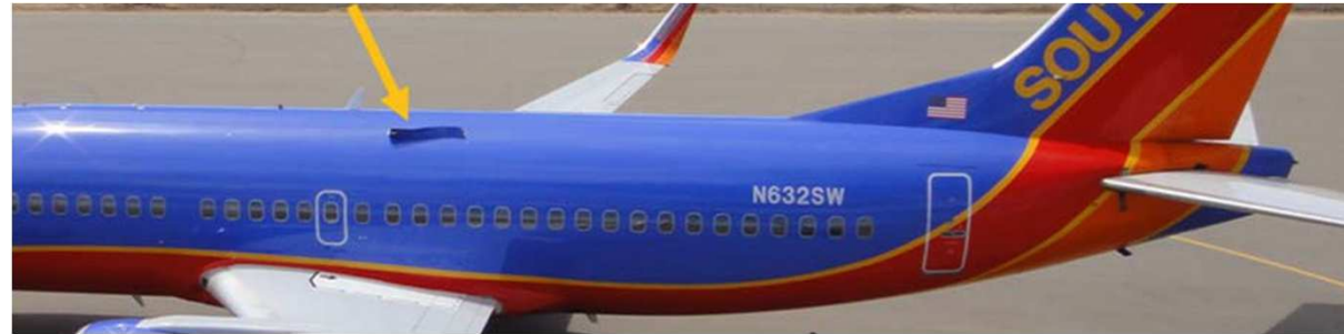
Structural failure of a lap joint in the fuselage skin due to metal fatigue cracks (Boeing 737, April 1, 2011)
